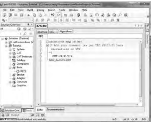
Figure 7-13 (a) Delete state INIT in ECC; (b) Modify algorithm REQ.
