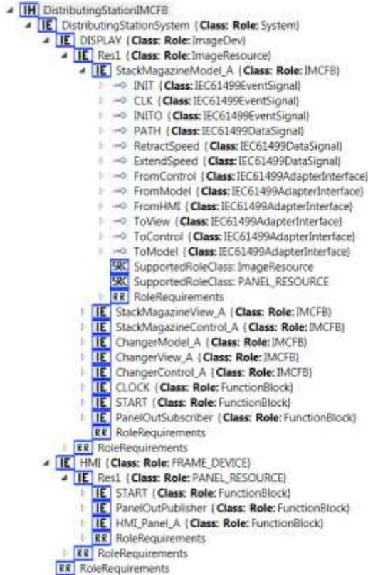
Fig. 14. InstanceHierarchy Template Example
