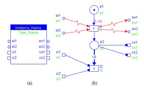
Figure 3 A Sample Basic NCES Module: (a) Module Interface, and (b) Module Content
