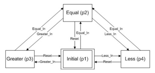
Figure 44 State Diagram of E\_Compare\_I
