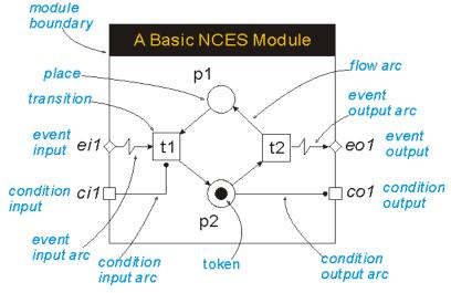
Figure 1 Graphical Notation of a Basic NCES Module
