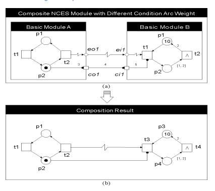
Figure 2 Composition of Composite NCES Module: (a) Original Module, and (b) Flatten Module
